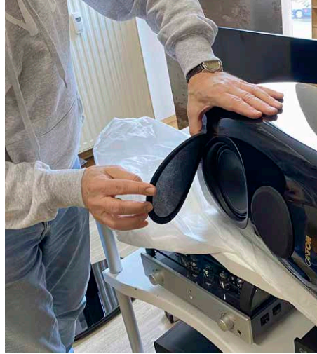
Each driver of the Reference 9 has its own asymmetrical and magnetically adhering dust cover.
